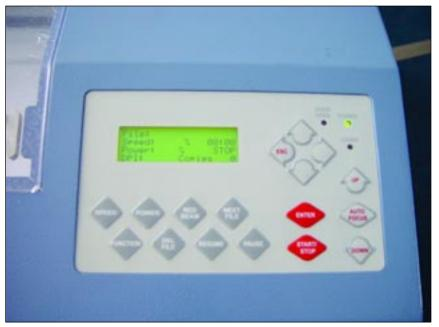
The control panel is simple and easy to use. The readout provides plenty of information about the job being engraved and the buffer allows for up to 99 jobs to be stored at a time.
