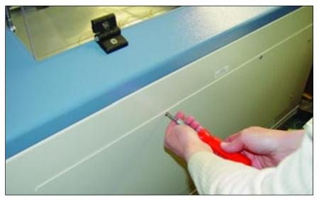
Removing eight screws from the back cover in order to use the pass-through capability is a reminder that this can be dangerous. Precautions should be taken when operating a laser with doors or panels removed.
