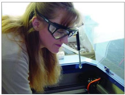
Special LaserShield glasses are a MUST when operating a laser when using the passthrough feature. These special glasses are provided with the laser.
